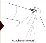
Attach your screen(s) to the 12 attachment points on the tube.
